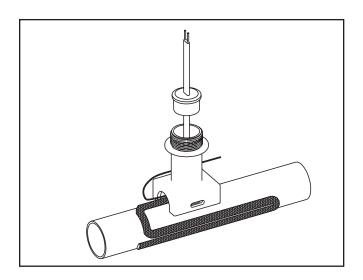
3. Insert cable though pipe standoff and grommet as shown. There should be 8" of cable past the grommets edge. Attach the pipe standoff to the pipe with a pipe strap (Chromalox type PS not included) as shown. Leave braid of the cable outside of pipe standoff and connect to ground (grounding clamp not included). Tape cable pipe as shown. For pipes smaller than 1 1/2" diameter a small pipe adapter (Chromalox model SPA not included) is required.
