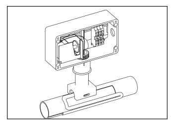
11. Assemble junction box to compression fitting as shown. Tighten locknut until the junction box bottoms out against the lip of the compression fitting. To ensure that box is water tight make sure washer for thermostat is against the enclosure.
