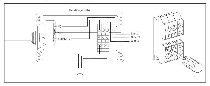
**12.** Attach 3/4" conduit hub. Use a flat head screwdriver to release the terminal spring clamps and insert cable leads and grounding braid. Please see the electric diagrams below for proper wiring for your application. Attach junction box cover to seal enclosure. **NOTE:** The conduit hub should be approved for Class 1, Div. 2; Class II Div. 1 & 2, Class III, Div. 1 & 2, and NEMA 4X rated by a nationally recognized testing laboratory.
