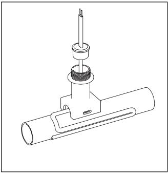
I. Insert heating cable and grommet as shown. 8" of cable should extend past the grommet. Attach the pipe standoff to the pipe with a pipe strap (Chromalox type PS not included) as shown. Attach extra cable to pipe as appropriate. For pipes smaller than 1-1/2" diameter optional small pipe adapter (Chromalox model SPA not included) is required.
