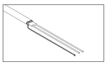
Remove the exposed core material and cut 1/4" of the end of each bus wire. \*Skip this step if using CWM-C constant wattage cable.
