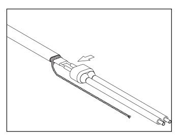
Liberally apply RTV over the exposed matrix and leads. Push the rubber boot over the heating cable. Trim lead ends as needed.
