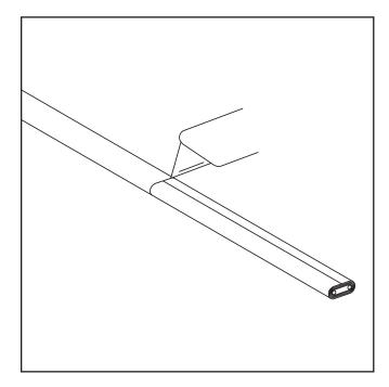
Score the outer insulation 7" from the end of the cable. Lightly cut the outer jacket up the center to the end of heating cable and remove the outer jacket from the cable. WARNING: DO NOT CUT METAL BRAID.
