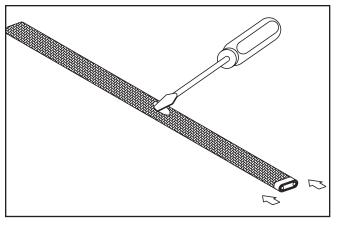
For each cable, push braiding back from the end of the cable. 11" from cable end create a bulge. At the bulge, separate the braid to make an opening.
