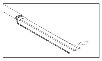
7. Starting at the end of the heating cable, using needle nose pliers or a knife pull each bus wire away from the core material.
