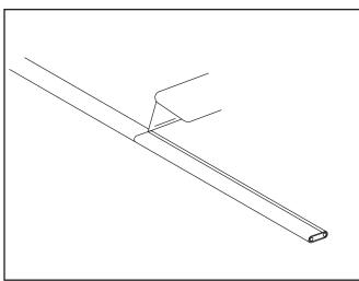
4. Score the inner insulation 7" from the end. Lightly cut the inner jacket up the center to end of heating cable and remove the inner jacket from the cable.
