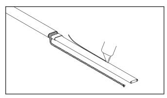
**6.** Shave the core material from the outside of each bus wire.
