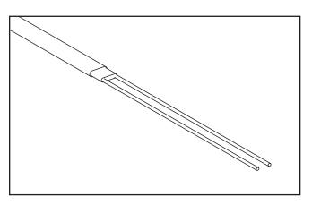
7. Remove the exposed core material and cut 1/4" off the end of each bus wire. \*Skip this step if using CWM-C constant wattage cable.
