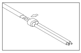
**8.** Liberally apply RTV over the exposed matrix and leads. Push the rubber boot over the heating cable. Trim lead ends as needed.
