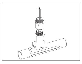
10. Slide compression fitting over cable. Grommet should be placed inside pipe standoff. Termination boot should be spaced 1/2" from sealing grommet. Tighten compression fitting until it bottoms out against pipe standoff.
