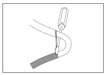
**4.** While bending the heating cable, work the cable through the braid opening. Pull the braid tight.
