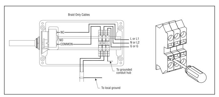
**11.** Attach 3/4" conduit hub. Use a flat head screwdriver to release the terminal spring clamps and insert cable leads and grounding braid. Please see the electric diagrams below for proper wiring for your application. Attach junction box cover to seal enclosure. Note: The conduit hub should be approved for Class 1, Div. 2; Class II Div. 1 & 2, Class III, Div. 1 & 2, and NEMA 4X rated by a nationally recognized testing laboratory.
