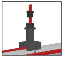
1. Insert cable without the braid through pipe standoff and grommet as shown. Attach pipe standoff to pipe with pipe straps (Chromalox model PS not included). Leave braid outside of pipe standoff at grommet. For pipes smaller than 1 1/2" diameter a small pipe adapter (Chromalox model SPA not included) is required.
