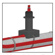
**4.** Adjust cable leaving 1" past the end of the grommet and insert the grommet into the pipe standoff. Attach extra cable to pipe as shown.
