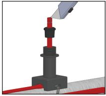
2. Score the outer insulation 1/2 inches from the end of cable. Lightly cut the outer jacket up the center to end of heating cable and remove the jacket from the cable.
