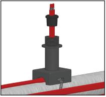
Using wire cutters trim exposed grounding braid away from the end of the cable.
