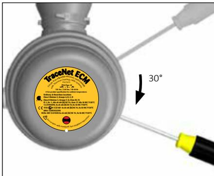
**21.** Install junction box lid and twist hand tight. Insert screwdriver into ratchet slot located on side of junction box base to tighten. Use screwdriver to ratchet on junction box lid. Lid will rotate 30° for tight seal. To remove lid, repeat step 21 in opposite direction.
