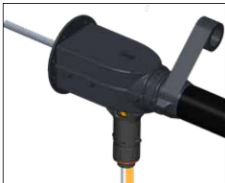
**12.** Apply self-vulcanizing tape around bundle jacket and work up over FAK ends.
