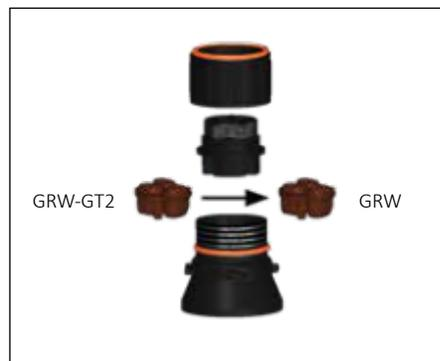
**11.** For HPT and FP cable, exchange grommet in Terminator with GRW-GT2 provided in PETK-3-ECM.
