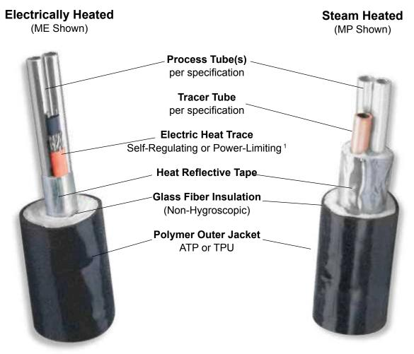
Standard TubeTrace Bundles are designed so the outer jacket will not exceed 60°C when the process tube is 204°C<sup>2</sup> and the ambient is 27°C, no wind.
