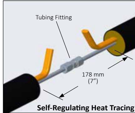
2. Cut 38 mm (1.5") off the end of the tubing and make tube fitting connections with appropriate fittings, provided by others. If no electrical heat trace is present, go to Step 4.
