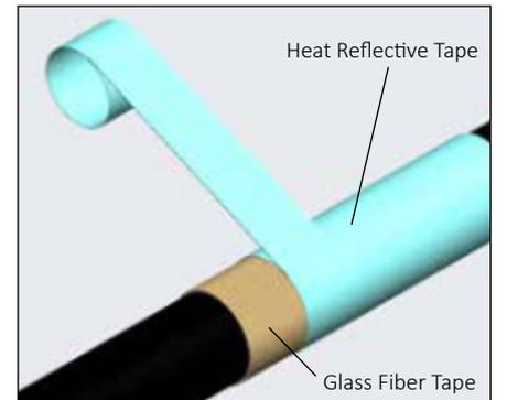
5. Complete with additional passes of heat reflective tape.
