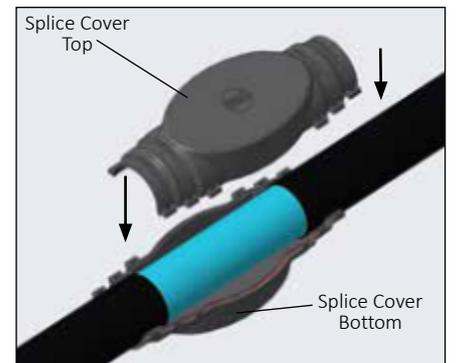
8. Fit tubing bundle to bottom half of cover and install top half. Snap together firmly. Inspect ends of tubing splice cover for snug fit. Apply additional RTV sealant where needed.
