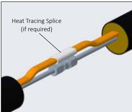
3. If bundle includes electric heat trace, make-up splice per instruction included with heat trace kit. This should be accomplished after fittings are leak tested.
